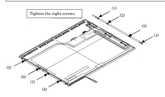
Figure 4-60 Replacing TMD fluorescent lamp (WXGA) (10)
